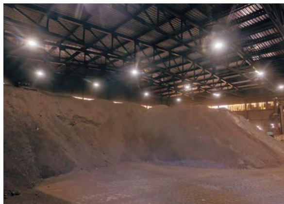
Waste from the automotive industry serves as the starting point for production. It is stored in a huge hall, mixed, and then prepared for the reduction units (image below).
